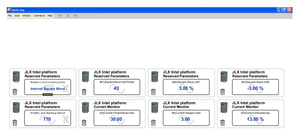
Parameter 860) Stator Current Commissioning Mode is the Savvy equivalent of the JL/X RESERVED MENU parameter Iarm COMMISSION.MODE. Note that the value displayed has now changed to Internal Square Wave.
