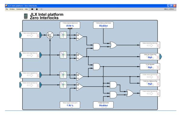
The threshold for Brake Engage Demand is set by 117)Zero Interlocks Speed Level.
