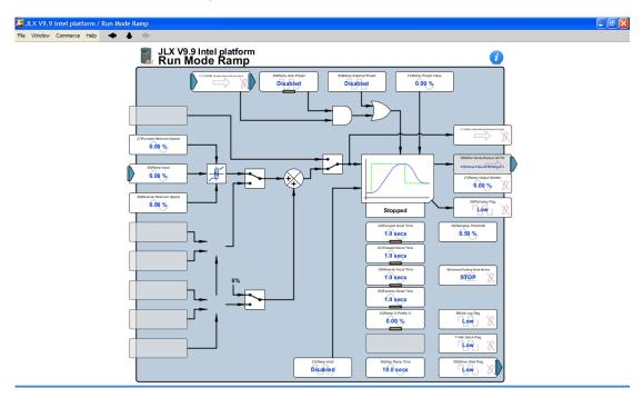
and restore any desired values in 22) Forward Accel Time, 23) Forward Decel Time, 24)Reverse Accel Time, 25) Reverse Decel Time and 32) Ramp S-Profile %.
