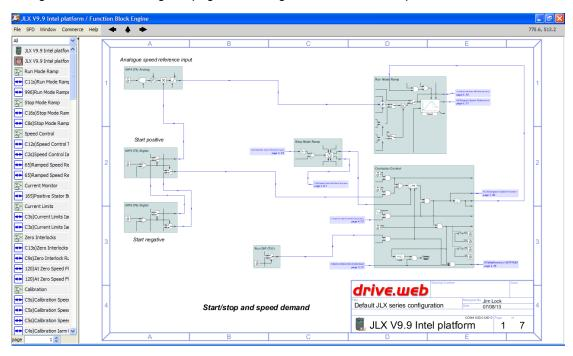
Navigate to the block diagram page containing the Run Mode Ramp block
