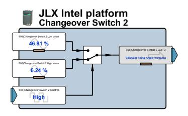
The stator firing angle minimum delay is set by 609) Changeover Switch 2 Low Value (when hyper-synchronous speed is demanded and achieved) and by 608) Changeover Switch 2 High Value under all other circumstances. The units are expressed as follows: (minimum delay \* 16384)/210 in degrees (only the integer number is taken, ignore the decimal places and % units). Thus the number for 60 degrees is (60 \* 16384)/210 = 4681, and the number for 8 degrees is (8 \* 16384)/210 = 624 for example.
