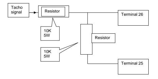
The example network shown will allow full speed voltages up to 400VDC whilst restricting the input terminal to 200VDC. The required setting for 8) Max Analog Tach Voltage is that at terminals 25, 26 at full speed. Appropriate measures must be taken to dissipate the heat from the dropper resistors. The total power in watts dissipated will be (Tacho signal volts)<sup>2</sup> / 20,000 in the example shown.
