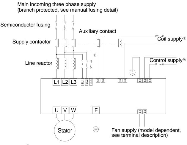
$^{*}$  Note: EL1,2,3 terminal wiring, control supply and coil supply breaker or HRC fuse protected
