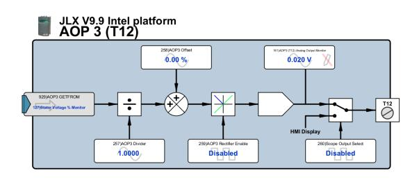
Delete the 929) AOP3 GETFROM connection and connect instead to 718) Unfiltered Current Demand Monitor. Also set parameter 257) AOP3 Divider to 2.0000.
