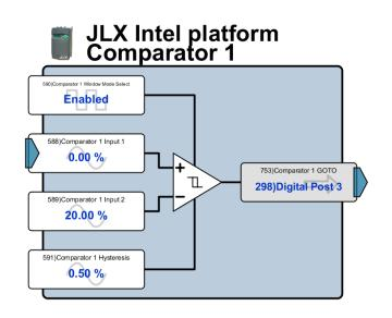
The Brake Release Authorisation stator current threshold is set by 589)Comparator 1 Input 2.
