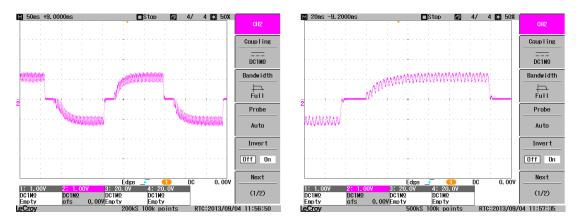
**Important note:** The maximum average level observed on the oscilloscope trace will be scaled according the ratio of your setting for 2) RATED STATOR AMPS against the maximum current capability of the JL/X model in use. The maximum will be 3V for 150% current on a JL/X set for its maximum current capability. For example, a setting for 2)
