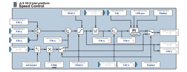
If necessary, reduce the value of 72) Speed Integral Time Constant so that the speed follows the step change in speed demand as closely as possible. Then return to the block diagram page containing the Speed Control block, left click on the Parameter Profiler block
