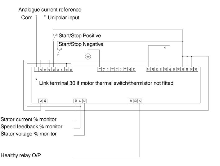
5.6 Basic joystick/digital input current control (3-key reset configuration).
