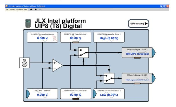
The positive hyper-synchronous detection level is set by 389)UIP8 Threshold. This in turn is set by 385)UIP8 High Value for Output 1 and 386)UIP8 Low Value for Output 1. The values for these parameters should be set symmetrically around the desired hyper-synchronous detection level in order to provide hysteresis. For example, a
