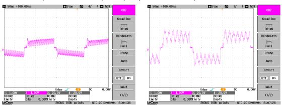
The next two pictures show examples of poorly tuned current loops.
