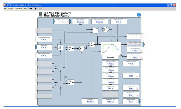
Set 22) Forward Accel Time, 23) Forward Decel Time, 24) Reverse Accel. Time and 25) Reverse Decel. Time to 0.1 seconds. 32) Ramp S-Profile % should be left at 0.00%.
