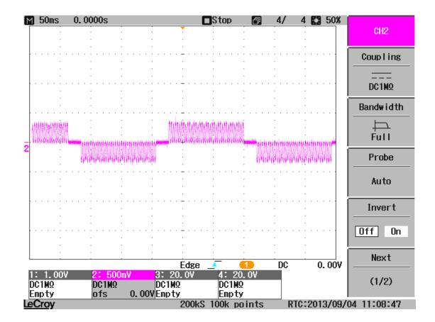
The next picture shows a close up of the zero current region as the JL/X switches bridges. There should be a "dead time" around zero current of around 18mS (on a 50Hz supply) as the following picture shows, but the "dead time" may well be shorter if the stator is highly inductive.
