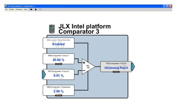
The threshold for DIO1 operation is set by 596) Comparator 3 Input 1, and hysteresis by 599)Comparator 3 Hysteresis.
