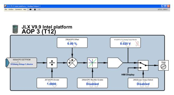
Delete the 929) AOP3 GETFROM connection, and connect it instead to 127) Stator Voltage % Monitor, which was its original configuration.
