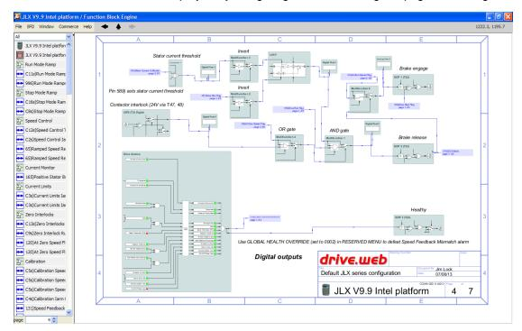
The available alarms can be displayed by navigating to the block diagram page containing the Drive Alarms block
