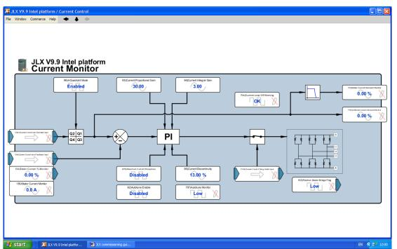
Set 678) Maximum Current Response to Enabled. It is now possible to set values up to 300 in 875) Min. Iarm Blanking Interval value.
